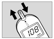
A test result may be deleted at the end of a test during the 3 minutes it is displayed. Use a tissue to pull out the Test Strip and quickly insert it back into the Meter (within 2 seconds).
